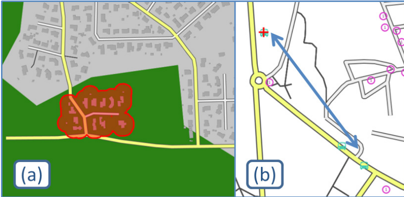
Fig. 12: (a) This automatically identified group of buildings should not be inside the forest. (b) The automatically identified bus stop (highlighted by the red cross) is too far from a road. ©OpenStreetMap contributors.
